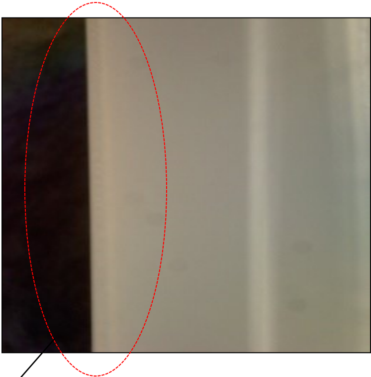
Melt fracture does not occur.
