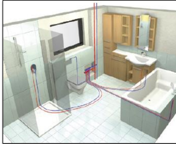
Plumbing (Hot & Cold water)
