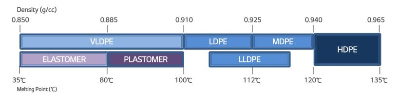
**Polyolefin elastomers(POE)** with densities between 0.857 and 0.885 are used in the manufacture of TPOs, which are used for automotive, recreational goods appliances, house-wares, and other miscellaneous applications.
