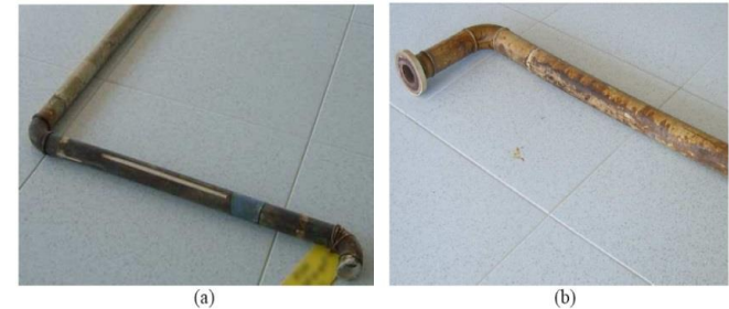
Fig. 1: Investigated samples: (a) Pipe-1/Fitting-1 operated with H_2SO_4 and (b) Pipe-2/Fitting-2 operated with CoCl_2 .
